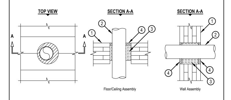
FIGURE 1. THROUGH PENETRATION FIRESTOP SYSTEM
