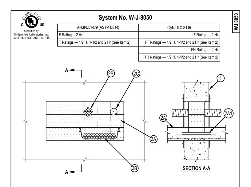
Wall Assembly — Min 5 in. (127 mm) thick reinforced lightweight or normal weight (100-150 pcf or 1600-2400 kg/m3) concrete. Wall may also be constructed of any solid or filled UL Classified Concrete Blocks\*. Max area of opening is 288 sq in. (1858 cm2) with max dimension of 24 in. (610 mm).
