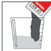
2. Important! First add clean water to separate container. Then slowly add CP 637 to water while stirring by hand or power mixer to ensure smooth, lump-free mix. See table above for mix ratio.
