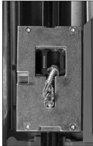
Jammed driving chamber
