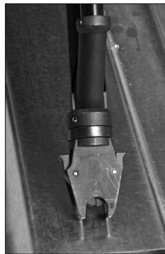
SDT 5 nose prior to first compression shows no screw loaded into the driving chamber
