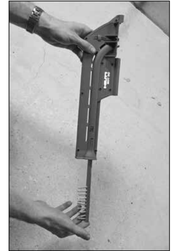
To remove fasteners, insert plastic strip and tilt magazine downward
