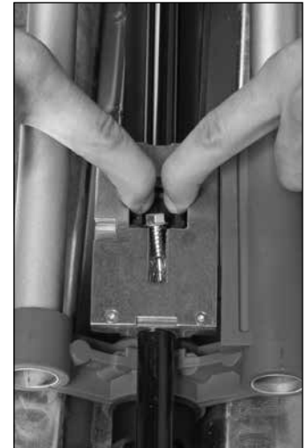
Opening the "teeth" in the feed area to release the jammed fasteners
