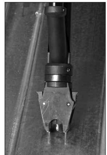
SDT 5 nose after first compression shows that tool is fully loaded and ready to begin fastening sidelaps
