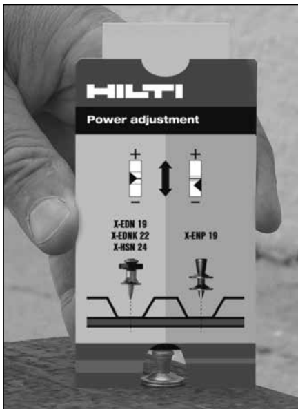
Under-driven X-ENP-19 (Guide stops in red zone - power adjustment necessary)
