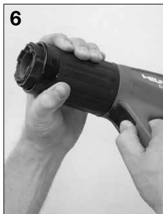
6 Remove the piston sleeve from the gas return unit by pressing down the button lock on the front of the handle
