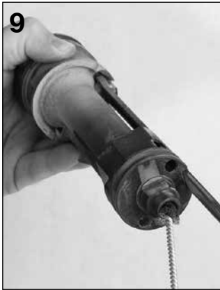
Brush combustion chamber
