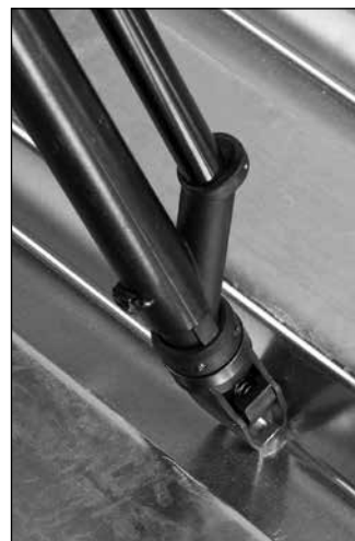
Use ridge of deck as backstop to minimize slipping
