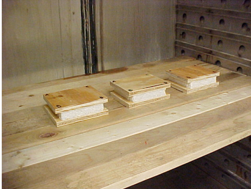
Photo No. 9 Dimensional Stability - Humidity Controlled Conditioning
