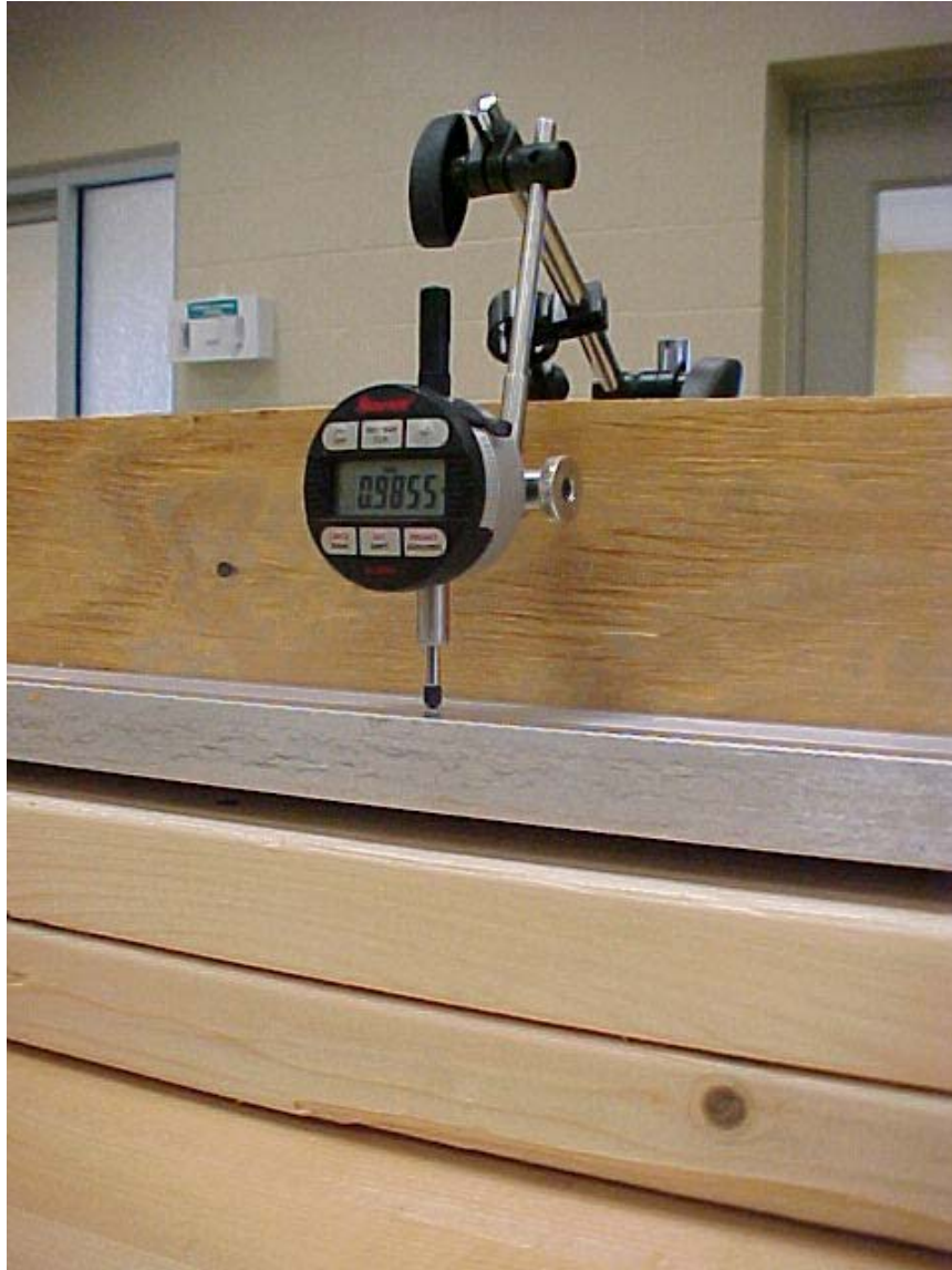
Photo No. 13 Beam Deflection Construct - Deflection Gauge
