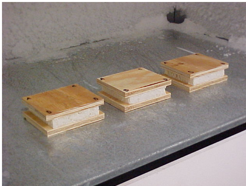
Photo No. 8 Dimensional Stability - Cold Conditioning
