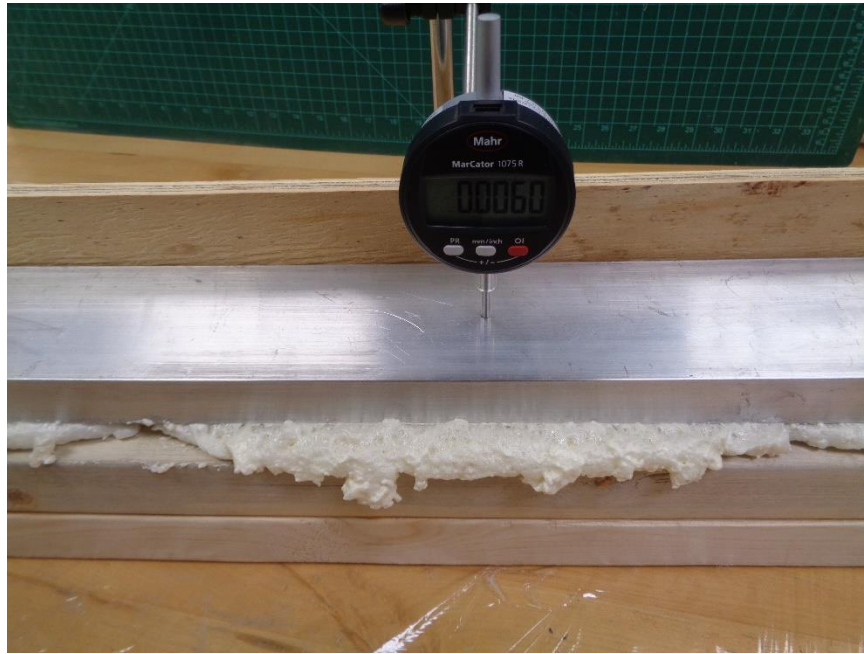
Photo No. 3 Beam Deflection Testing
