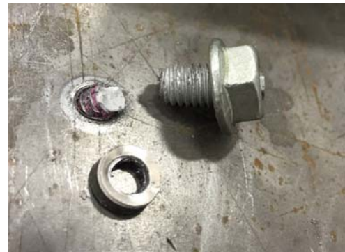
Figure 8 - Typical Fastener Shear Fracture Failure
