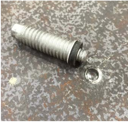
Figure 5: Typical Seismic Tension Failure – Fastener Pullout
