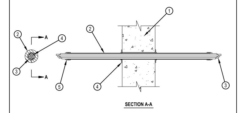
1. Wall Assembly — Min 6 in. (152 mm) thick reinforced lightweight or normal weight (100-150 pcf or 1600-2400 kg/m3) concrete Wall may also be constructed of any UL Classified Concrete Blocks\*. Max diam of opening is 1-1/4 in. (31 mm).
